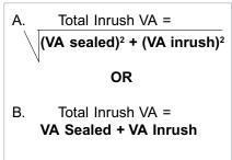
Note: method B will result in a slightly larger transformer being selected.
